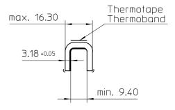
Dimensions in mm/inch and degrees Source: mm
